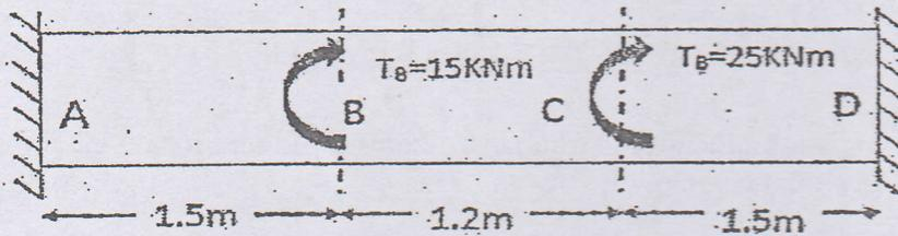
5. a) Determine the maximum bending stress in the beam shown in figure below. [10]
