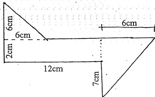
3. The state of stress in a two dimensionally stressed body is as shown in figure below. Determine principal stresses, principal planes and maximum shear. Determine also the normal and tangential stresses on plane BE and verify the results by drawing Mohr's circle. [16]
