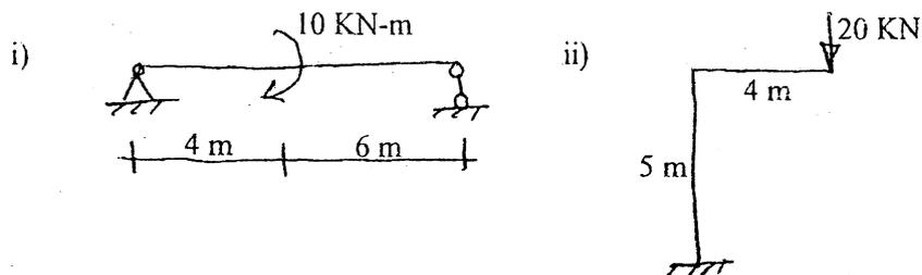
b) Draw axial force, shear force and bending moment diagram for the frame shown in figure below. [12]
