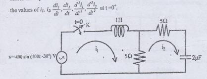
2. a) Using classical method, find the expression for the current supplied by the source in the network shown in figure. Also find the time taken by the source current to reach 25 mA.
