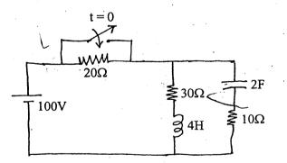
b) At t = 0, switch is closed in the circuit of figure below. Find the V<sub>c</sub>(t) and i<sub>c</sub>(t) using classical method.
