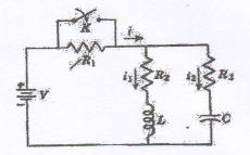
4. a) Find the forward voltage ratio transfer function  $G_{21}(s)$  and forward transfer admittance  $Y_{21}(s)$  in the following circuit.
