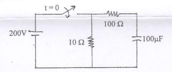
b) Keeping the switch closed for a long time, if the switch is opened at t = 0 in the circuit shown in figure below, find expression for voltage across capacitor using classical method of solution.
