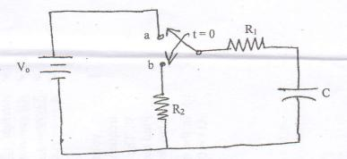
b) Using Laplace Transform method in the circuit shown in figure below. Find the current  $i_1$  and  $i_2$  for t > 0.
