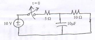
b) After being closed for a long time, if the switch in the circuit shown in figure below is opened at t = 0. Obtain the expressions for  $i_L(t)$  and  $v_c(t)$  for t > 0, using Laplace Transform Method.
