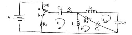
b) Switch in the circuit is suddenly opened at t = 0 after steady state has been reached in the closed position of the switch. Use classical method to determine the expression for voltage across capacitor for t > 0.
