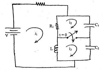
b) For the circuit shown in following figure, use classical method to find the current in the inductor for t>0.
