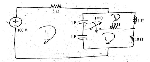
2. a) Find  $v_a(t)$  for t > 0 in the figure below using classical method.
