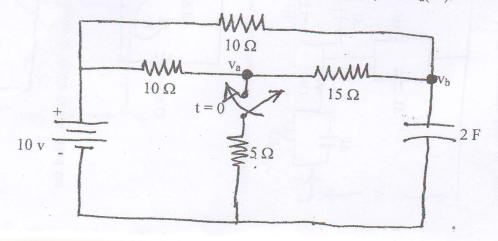
2. a) Using classical method in the circuit shown in figure below. Find the voltage across capacitor for t > 0.
