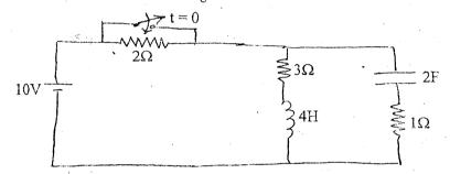
2. a) In the two mesh network shown in the figure below, the switch is closed at t = 0. Find the mesh currents  $i_1(t)$  and  $i_2(t)$  as shown, and the capacitor voltage  $v_C(t)$ . [Use classical approach].
