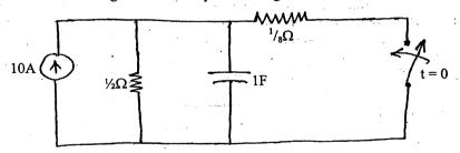
b) In the network shown, the switch is closed at t = 0. Find the current supplied by the source using Laplace transform method.
