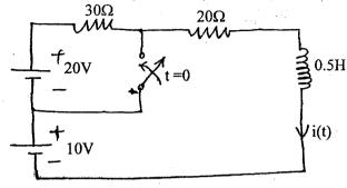
b) Using Laplace transform method, find the current  $i_1$  and  $i_2$  for t > 0 in the circuit of figure below.
