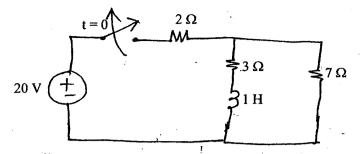
b) Using Laplace transform method, find he loop currents  $i_1$  and  $i_2$  for t > 0 in the circuit shown in the following figure. [8]
