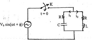
2. a) In the given circuit, after the switch has been in the open position for a long time, it is closed at t = 0. Find the voltage across the capacitor using classical method.
