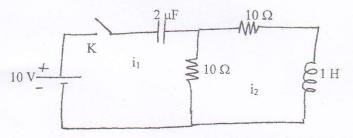
2. a) In the circuit of the figure below, the switch K is open and the circuit reaches a steady state. At t = 0, K is closed. Find the current in the inductor t > 0. Use classical method.
