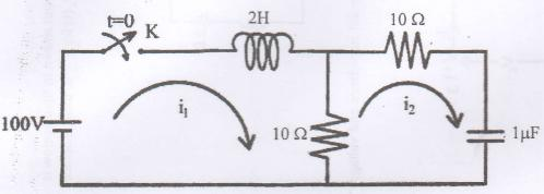
a) In the circuit shown in figure below, if the switch is closed at t = 0, find the expression for voltage across capacitor using classical method.
